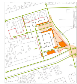
New extended public and semi-public space to boost commercial activity for the site (light orange). Pedestrian pathways network (green). Ground floor commercial units interact with newly created public space (orange).
