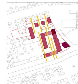
Building heights and orientation. While density is concentrated along the east side of the complex, the lower, east-west oriented buildings (C1, D2) allow sunlight to enter the courtyards. To the north, detached buildings (B1,2,3) allow sunlight, air and views to pass through to the neighbouring plots.
