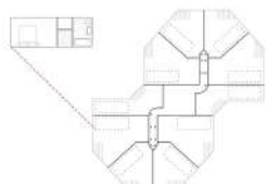
Standardized rooms, bathrooms, storages and kitchen units => reduced building cost
