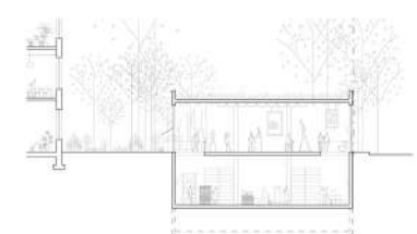
PARKING, FINAL STAGE - CROSS SECTION 1:200 Adaptive reuse: the floor between 2 and 4 is dismantled to create a 5 m high space for ateliers, production spaces etc; recovering natural light through voids opened in the ground floor.
